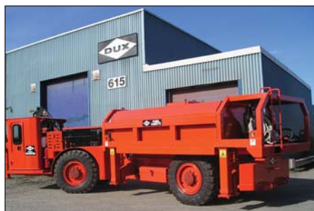
FUEL CASSETTE ATTACHED ON S1-PORTER
